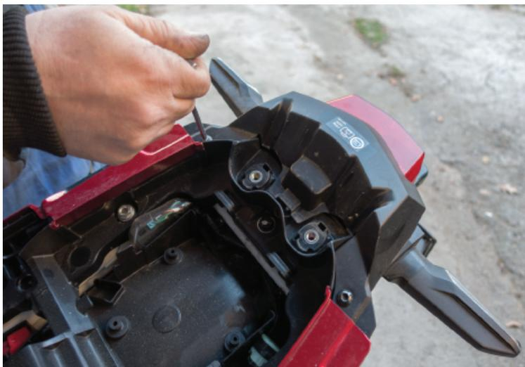
4. Gently remove the plastic cover without breaking the small clips.
