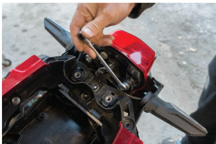
6. Using a 5mm Allen key, remove both Allen bolts that are in line with the rear turn signals.
