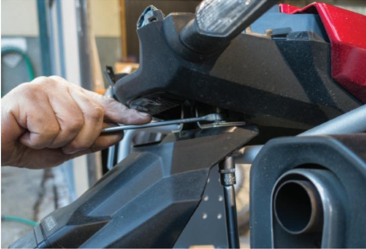
16. Re-insert the top middle bolt you removed in step #7. Tighten it.
