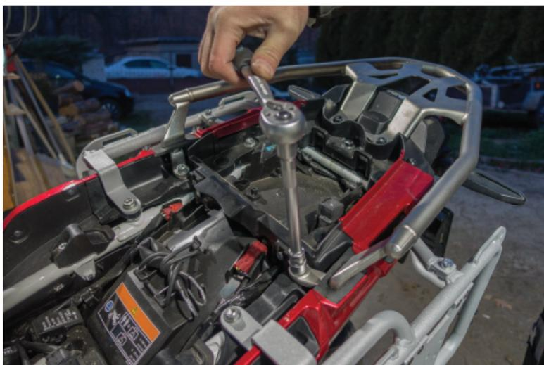
**22. Finally tighten all the bolts and nuts. Make sure to double-check all the bolts and nuts once again after a test ride.**
