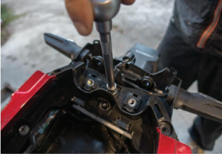
8. Remove both bolts from under the rear fender using a 12mm socket and wrench.
