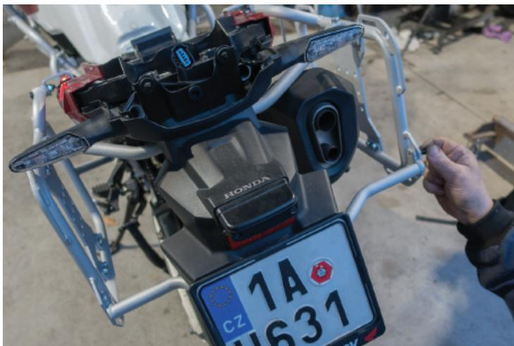
20. Re-install the rear brake light and the plastic cover.
