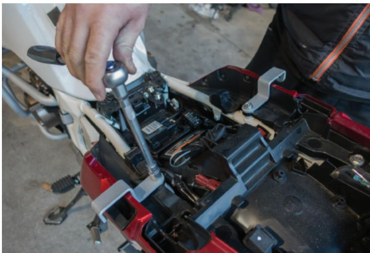
10. Remove the right side passenger foot peg. Between the front tab and the subframe, add the supplied spacer.
