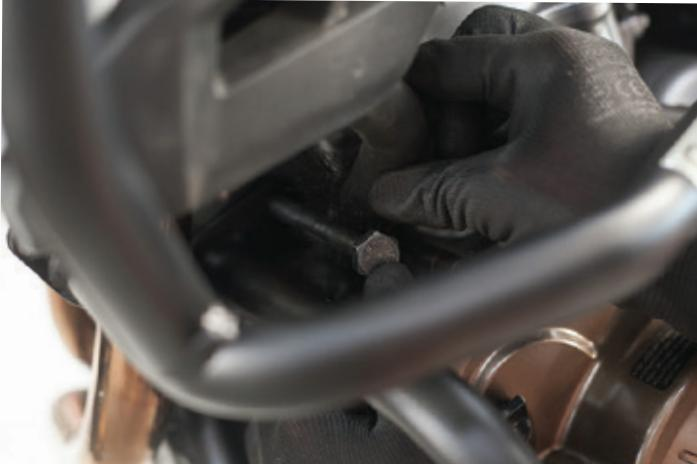
4. Mount the counterpart of the clamp on the reinforcement bar. Insert the two supplied button head Allen bolts. Place on the washers and hand-thread the nyloc nuts.
