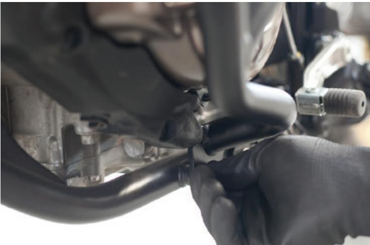
6. Move onto the right side (exhaust side) of your Africa Twin. Look underneath the bike. There are two through bolts in the frame.
