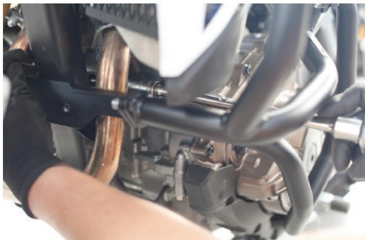
14. Repeat the same on the bottom through bolt using 13mm socket and wrench.
