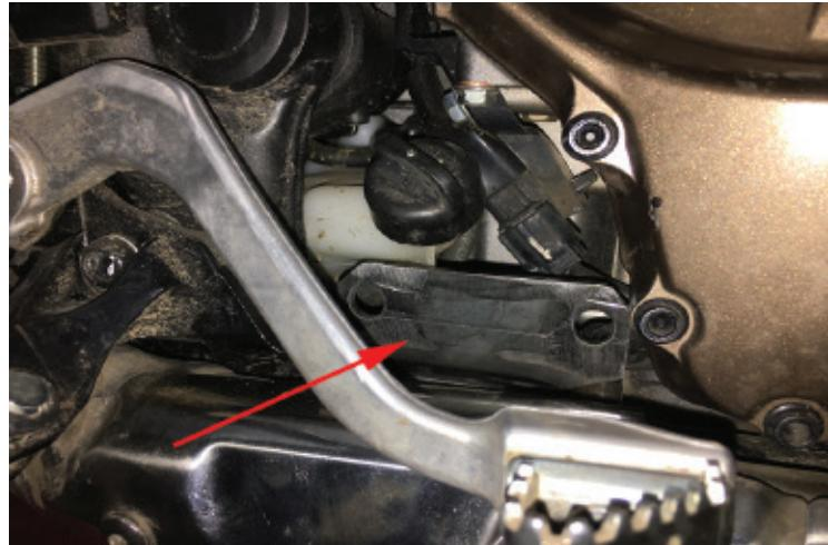
8. With the rear mounting tab now in place begin hand-threading the supplied flat nut (Part No.7.) on the front through bolt.
