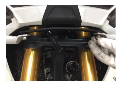
10. Finally, go ahead and tighten all the bolts and nuts to torque specs and make sure to check again after going out for a test ride.
