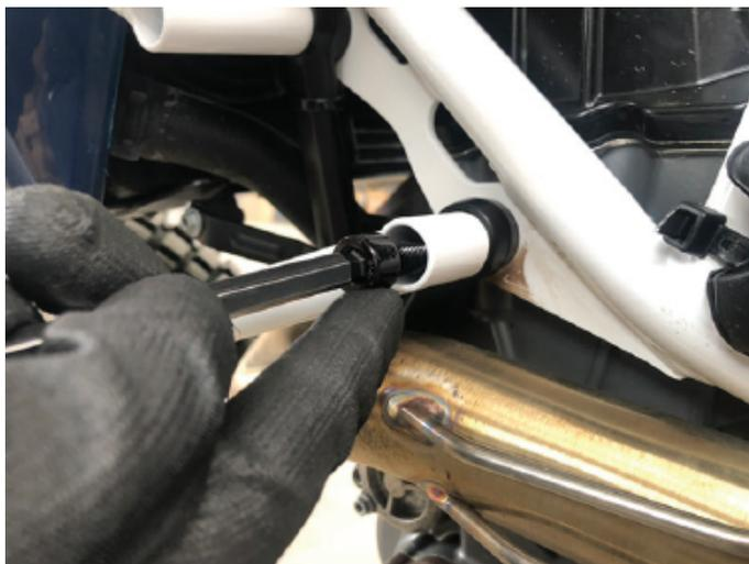
6. Remove the lower factory Allen bolt on the right side of the motorcycle.
