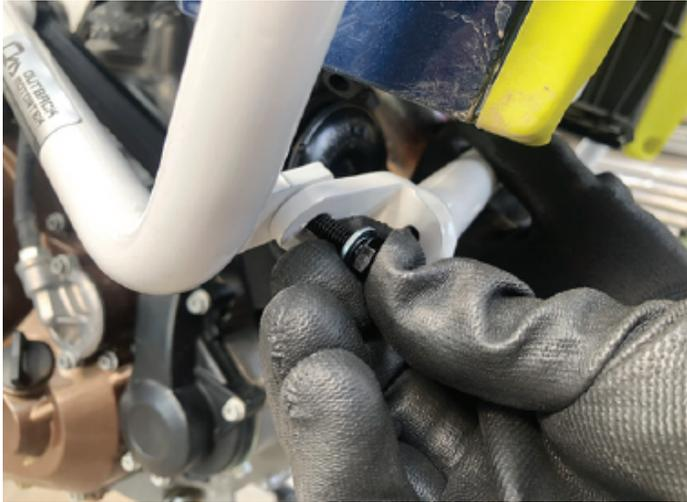
12. Then hand-thread the supplied locking nuts. Use 2x 10mm spanners/wrenches to tighten.
