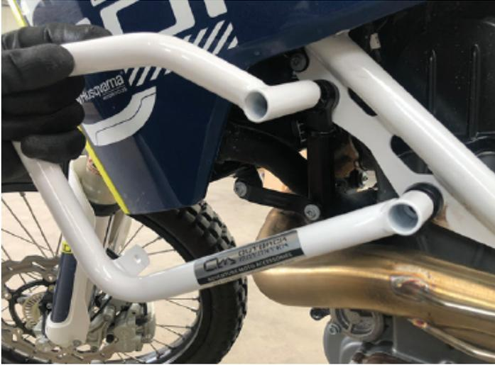
4. Insert the supplied M10x30mm bolt on the top. Only one or two turns to keep the bolt loose.
