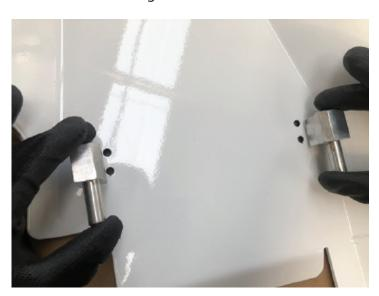
6. Hand thread the supplied M6 Allen bolts through the bottom.
