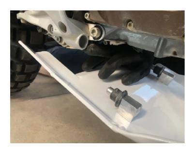
10. Hand thread the supplied M6 hex/torx bolts after lining up the mounting holes on the skid plate and the frame mounted bracket. Tighten the bolts using 10mm socket or wrench or torx key.
