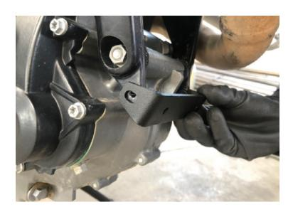
2. Secure it on the frame's mounting points by hand threading the supplied hexagon head bolts on both sides.
