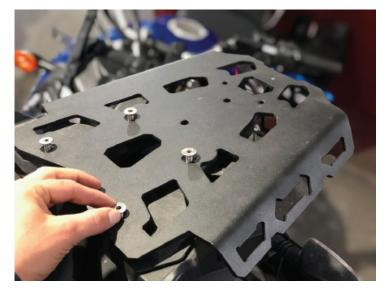
4. Take a 5mm Allen key or Allen socket and a ratchet and tighten down all four bolts.
