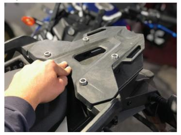
2. Next, take the rear luggage rack and gently put it on top of the four spacer. Make sure the mounting holes all line up.
