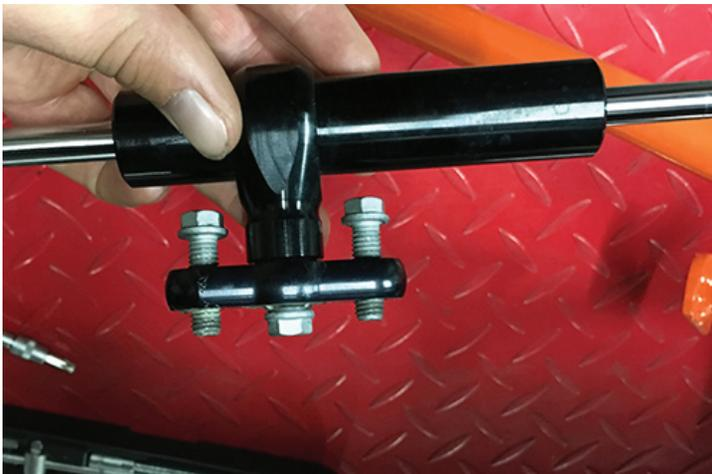
6. Hand-thread the left side factory bolts back into the frame mounting points. Do not tighten it, yet.
