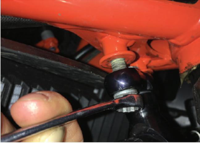
4. Mount the supplied bracket. Line up the bottom mounting holes with the factory crash bars' holes and insert the supplied M6x30mm bolts.
