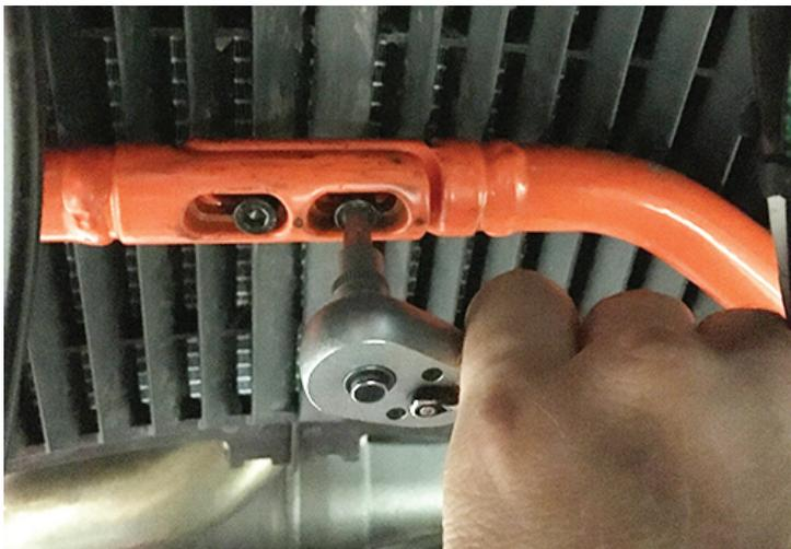
2. Remove the factory steering dampers using either a 10mm socket or T40 torx.
