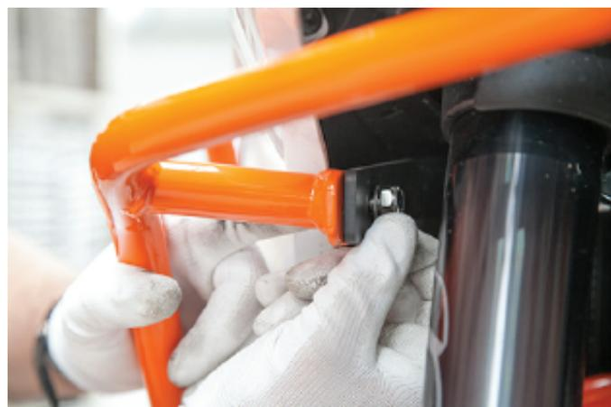
10. Next: take one of the "C" shaped clamps and two of the M6x30mm bolts+washers and nyloc nuts and secure the front lower part of the upper crash bars onto the factory lower crash bars.
